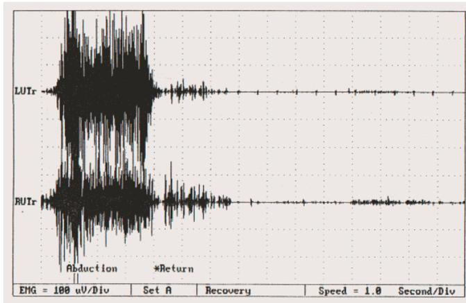
The x-axis displays time and the y-axis displays amplitude in  $\mu\text{Vs}$  (microvolts).
