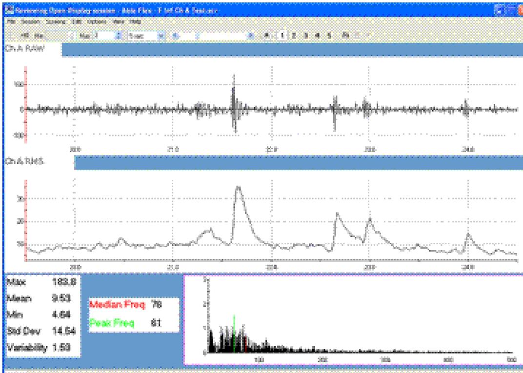
This biofeedback screen shows a Raw Line graph, RMS Line Graph, Max, Mean, Min, Std Deviation, Variability stats, and Median and Peak Frequencies and a 2D power spectrum.
