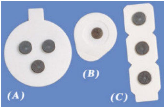
(A) Triode, electrode with standard 2cm spacing of silver-silver chloride electrodes, backed with nickel plated brass snaps to prevent corrosion when connected to pre-amplifiers for extended periods.
