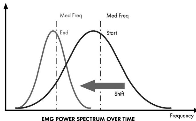
**Figure 3.** As a muscle fatigues, the power density spectrum and the frequency spectrum shift to the left side of the frequency scale, and consequently, the median and mean frequencies decrease. Note that mean and median frequencies are relevant muscle fatigue indicators only for isometric contractions (sustained contraction with no movement). Graphic courtesy of [www.thoughttechnology.com](http://www.thoughttechnology.com).
